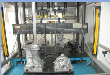
SMART MECHATRONIC CONTROL SYSTEM FOR IN VACUUM TIGHTNESS CONTROL OF MACHINED R145 CARTERS
