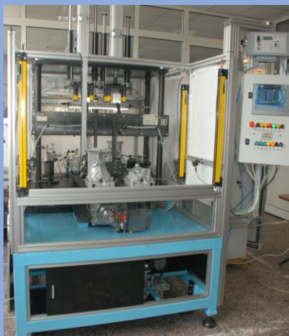
SMART MECHATRONIC CONTROL SYSTEM FOR IN VACUUM TIGHTNESS CONTROL OF MACHINED R145 CARTERS
